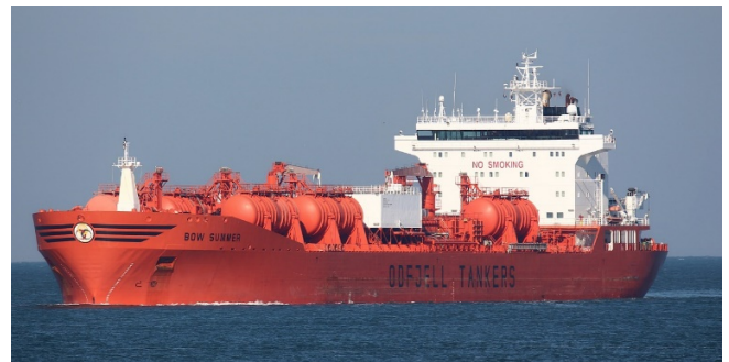
Odfjell's M/V Bow Summer. A Norwegianflagged chemical tanker with 40 separate tanks. Photo: Odfjell
